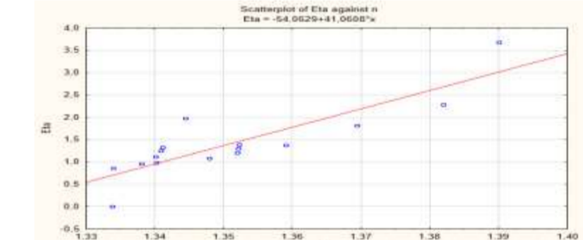
Regression line of dynamic viscosity ( \eta ) as a function of refractive index n
